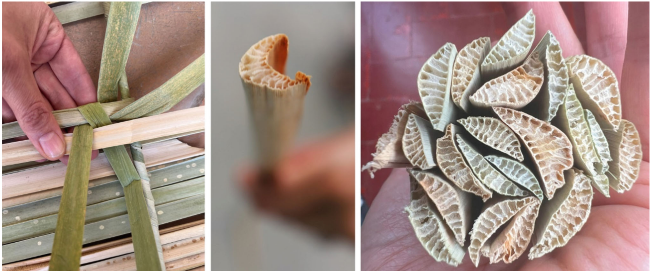
Fig. 5 Pliability of chuspata (left), linear rigidity (center), cellular structure (right). Photos by authors
